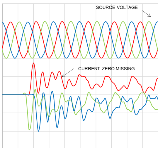
Figure 201 : Current zero missing phenomenon
